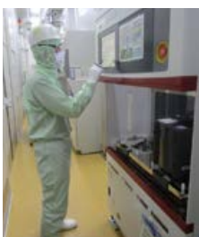
Inspection of the batch-type vertical film-forming system
